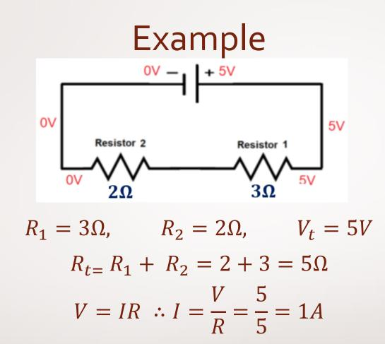
Now we can use Ohm's Law again to calculate the voltage drop in each resistor  $V_1 = IR_1 = 1 \times 3 = 3V$  and  $V_2 = IR_2 = 1 \times 2 = 2V$
